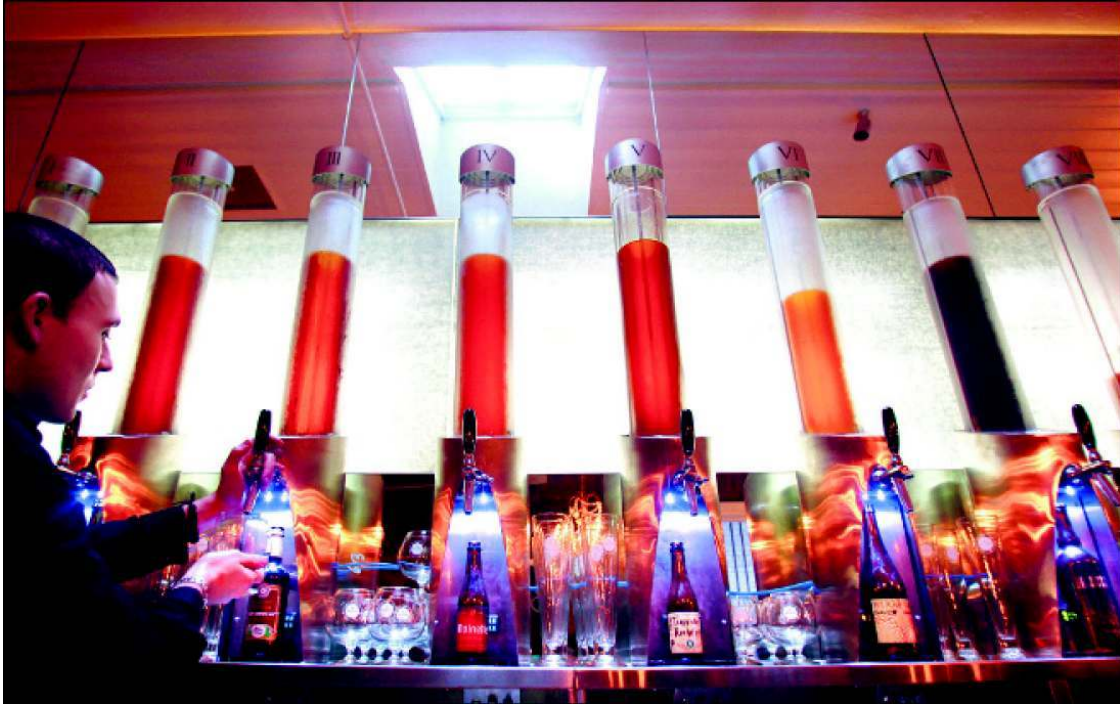
Biero's concept "beervault": The vaults allow bottled beer to be transferred into pressure and temperature-controlled tubes that act like kegs to keep beer fresh.
